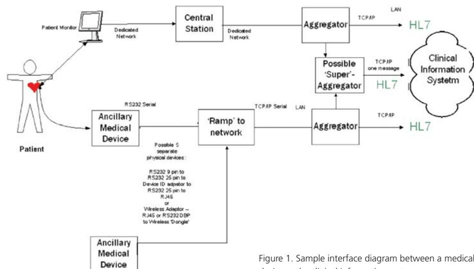
Figure 1. Sample interface diagram between a medical device and a clinical information system.
